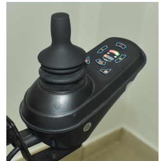
The control handle directs the wheelchair's movement.
