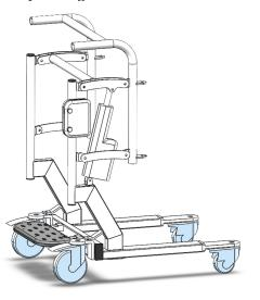
• 4. Install the left and right seat - back assemblies onto the corresponding mounting plates of the support tube assembly respectively, and lock them after passing the long screws through.
